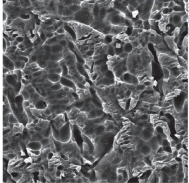
**Fig 1b** SEM image (2000X) of the HF-etched ceramic surfaces after ultrasonic cleaning in distilled water.
