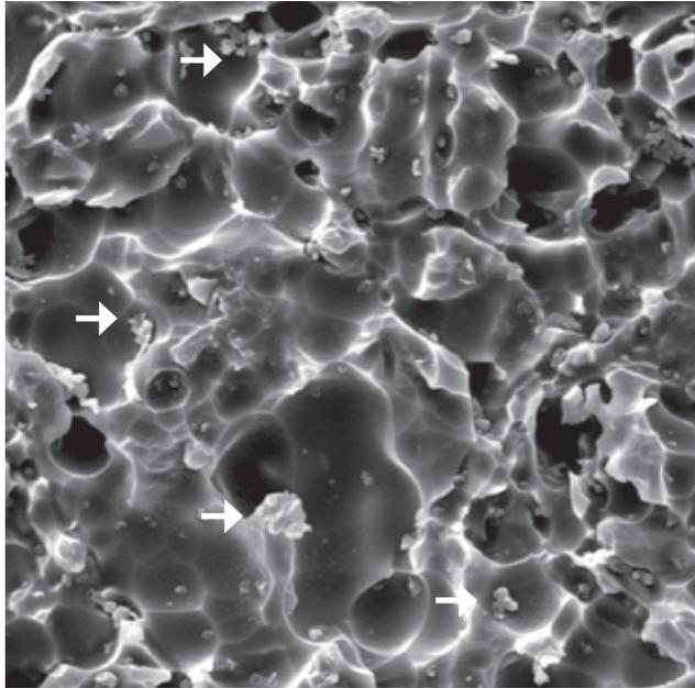
**Fig 1a** SEM image (2000X) of the HF-etched ceramic surfaces after air-water spraying. Note the precipitates after air-water spraying indicated by arrows.
