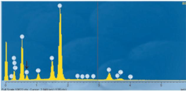
**Fig 2a** EDS analysis of the HF-etched ceramic surface after air-water spraying. Note the presence of F on the ceramic surface in the EDS analysis after water-spraying indicated by the arrow.
