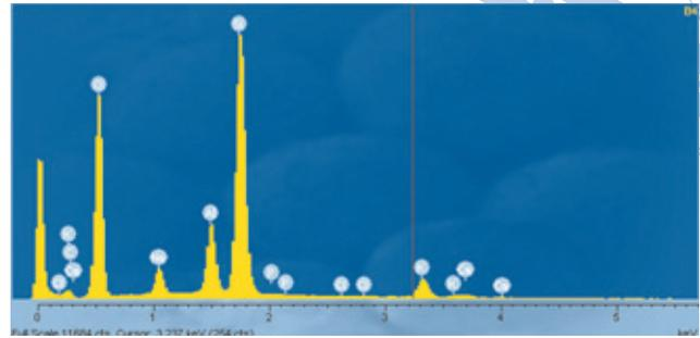
**Fig 2b** EDS analysis of the HF-etched ceramic surface after ultrasonic cleaning in distilled water. Note absence of F on the ceramic surface after ultrasonic cleaning in distilled water.
